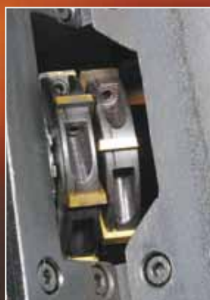
2 milling disks coupled with 6 indexable inserts each
